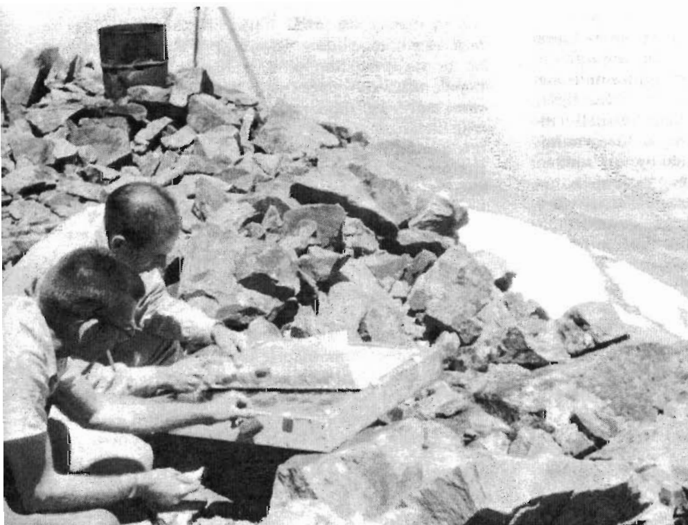
Left: Wade Patterson, Lawrence Laboratory, Berkeley, and his brother, removing sheets of gold foil from between layers of cadmium and paraffin to examine them for cosmic ray tracks. Summit Laboratory. August, 1958.
