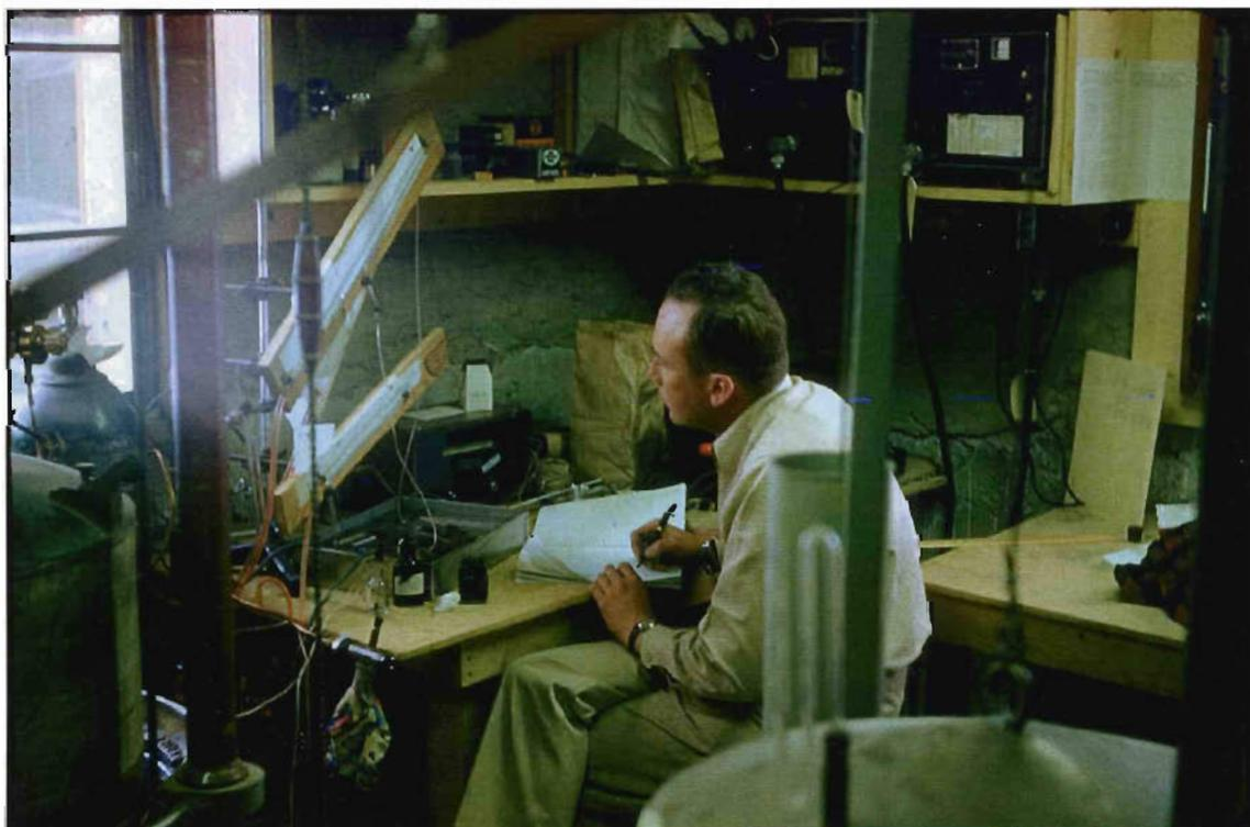
(*Left*) Determining ventilatory (respiratory) response to carbon dioxide; Ralph Kellogg is checking standardizations of gas mixtures, inside the Summit laboratory (14, 246 ft).
